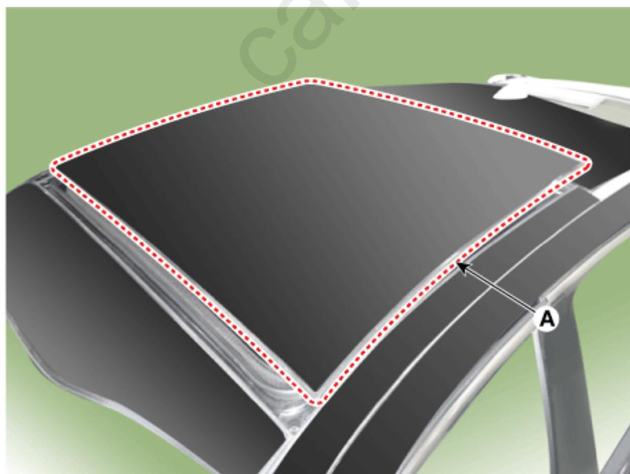
3. Remove the both sides mechanism cover (A).
