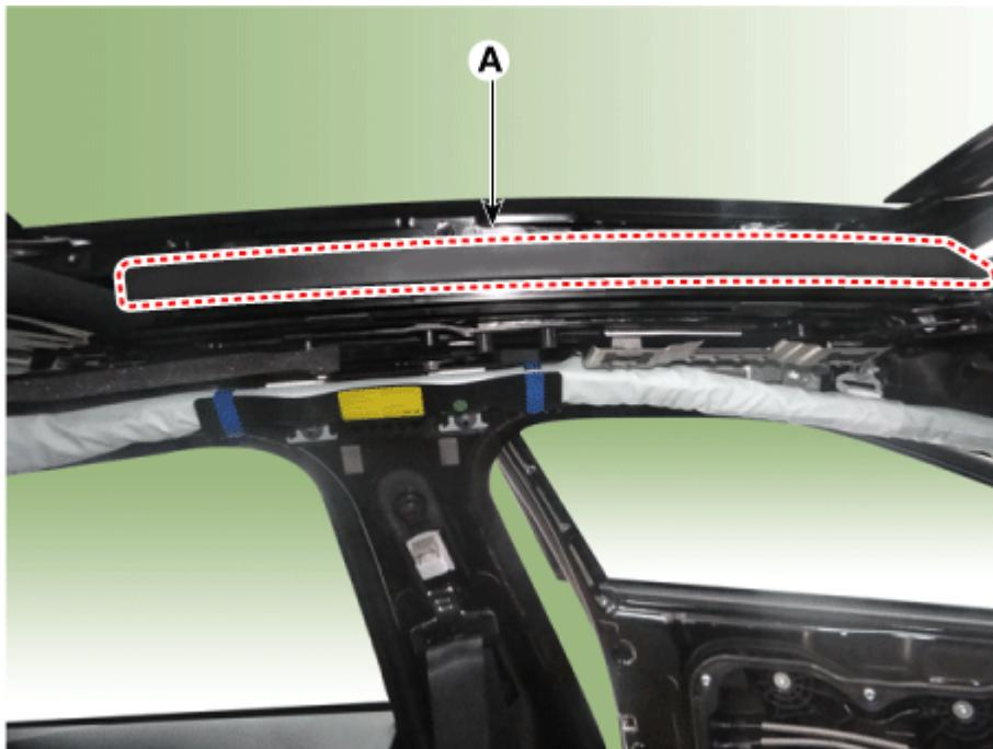
4. Adjust the height of the glass by slightly loosening the screws (A).
