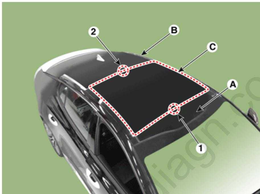
2. Tilt the moving glass by using the wide sunroof switch.
